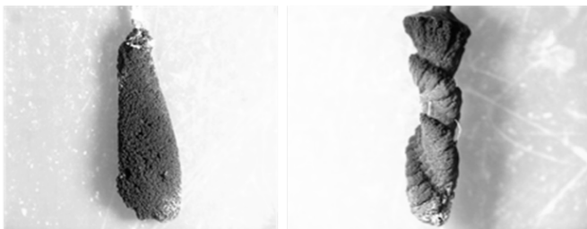
Fig. 1 Polythiophene deposits prepared at 0 T (left) and 4 T (right).
