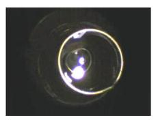
Fig. 2. A water thin film ( $\phi$ =ca. 25mm) on a copper ring prepared under quasimicrogravity.
