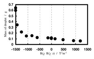
Fig. 1. Plot of water drop weight vs. BdB/dz.
